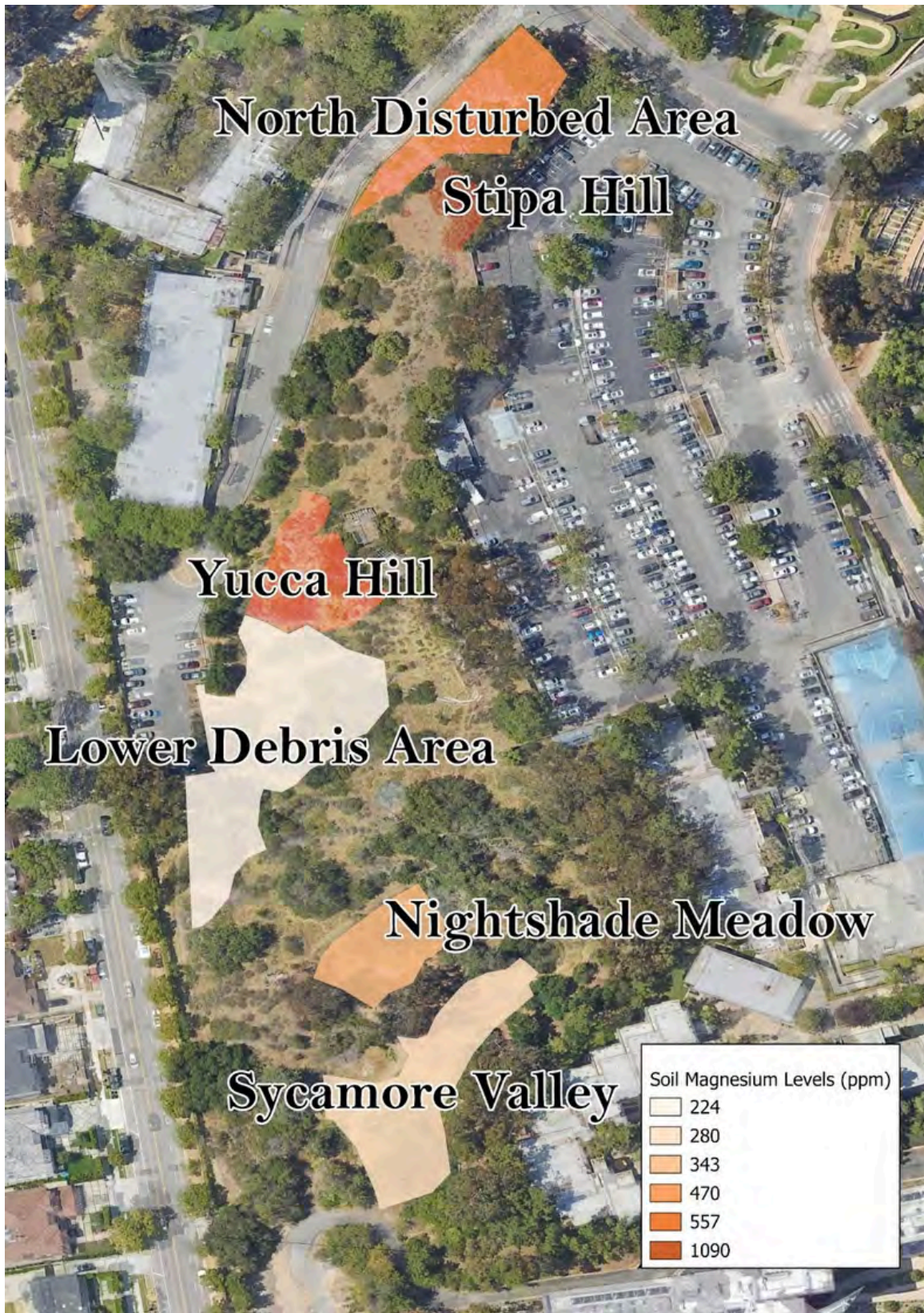
Figure 27: Soil Magnesium (Mg) Map with six sites colorized by varying levels of Mg in units of ppm.
