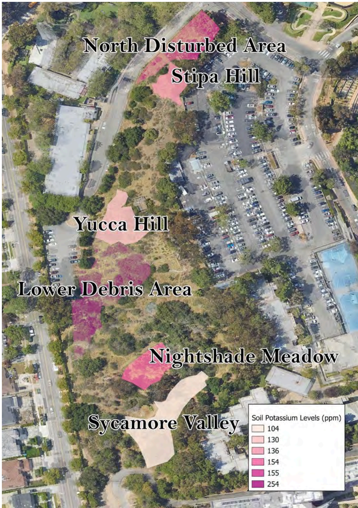
Figure 30: Soil Potassium (K) Map with six sites colorized by varying levels of K in units of ppm.
