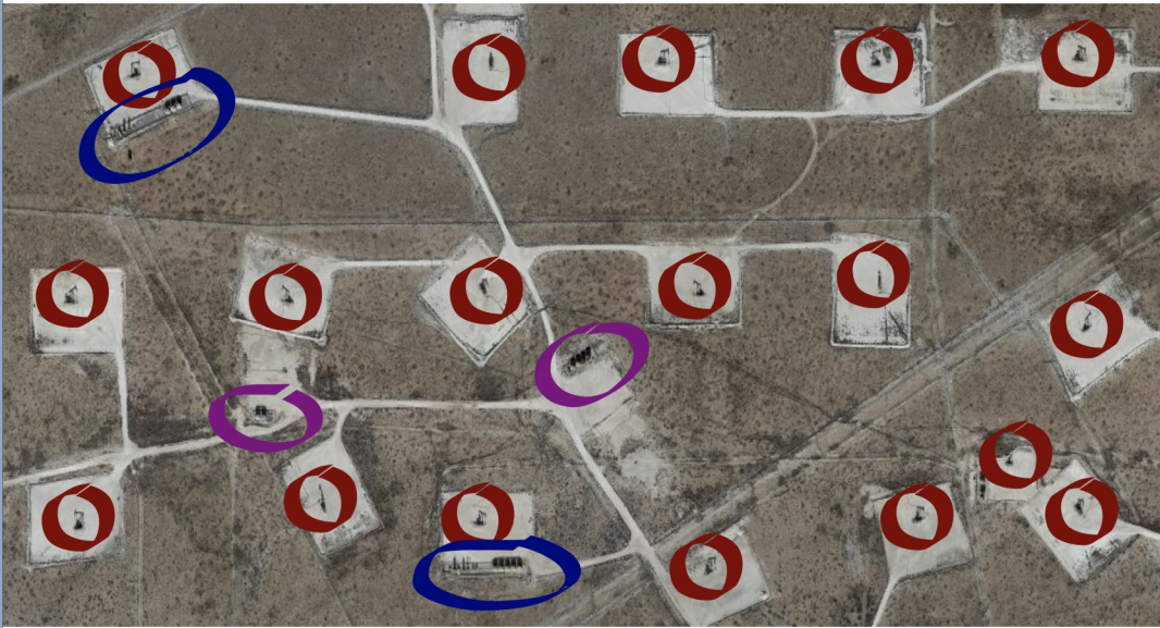
Figure 9. Aerial photo of oil and gas well distribution in the Permian Basin; the red circles are single wells, the blue circles are permitted facilities, and the purple circles are storage tanks (Google Earth).
