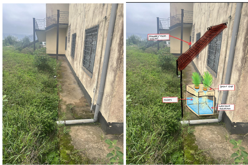
Figure 13 Location and proposed design of hydroponics system.
